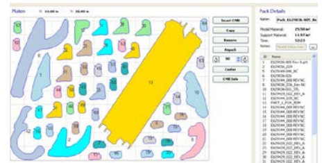
The Fortus 3D Production System's build tray size allows Western Tool & Mold to print different parts in different sizes in one go.
