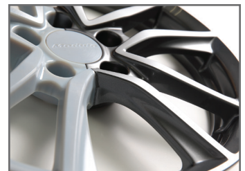
Wheel prototype model printed by Objet Eden500V: divided into few pieces and assembled.
