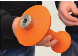
Volvo Trucks 3D printed this durable, lightweight punching tool on a Fortus 3D Production System.
