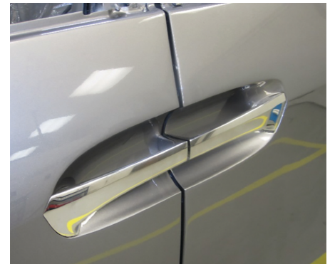
Final CNC machined prototype integrated into vehicle.
