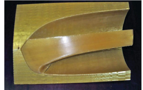
3D printed prototype of new design used to assess styling, fit and finish.
