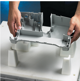
Oreck uses additive manufacturing to produce custom assembly pallets. During assembly, a vacuum top cover is placed into the pallet upside down.
