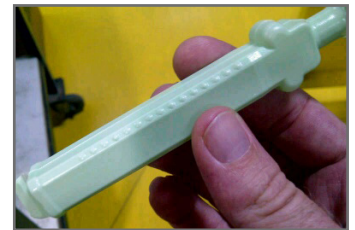
A PolyJet mold was used to produce 100 blow molded package prototypes.
